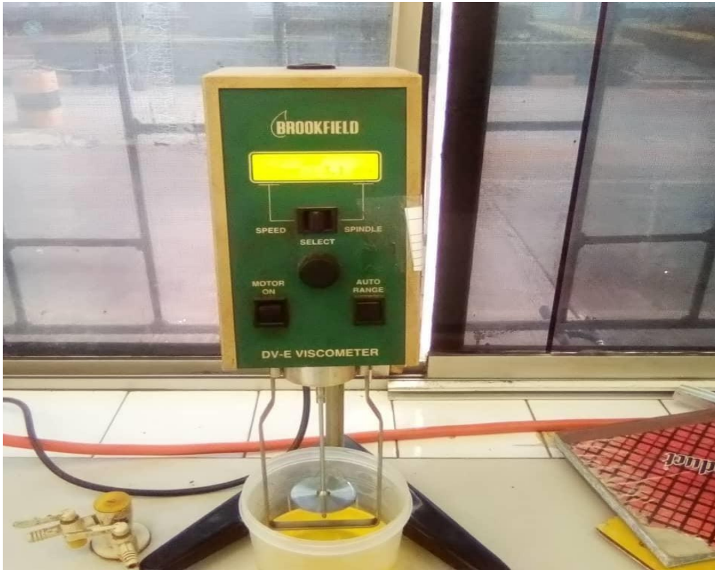
Figure 1: The DV-E Brookfield viscometer used for experimental measurement of oils viscosities.
