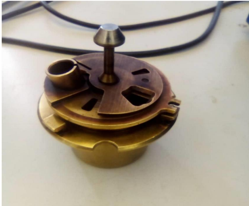
Figure 3: The flash point cup inside the PM-4 Petrotest flash point machine used for housing the spinning fluid Determination of the Oil Moisture Content
