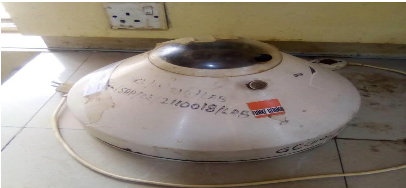
Figure 5: The FUNKE-GERBER Centrifuge Machine used in the determination of sludge
