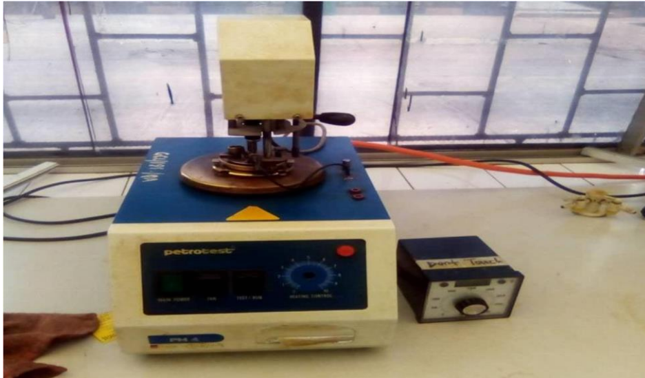
Figure 2: Experimental setup for flash point measurement using the PM-4 Petrotest flash point machine
