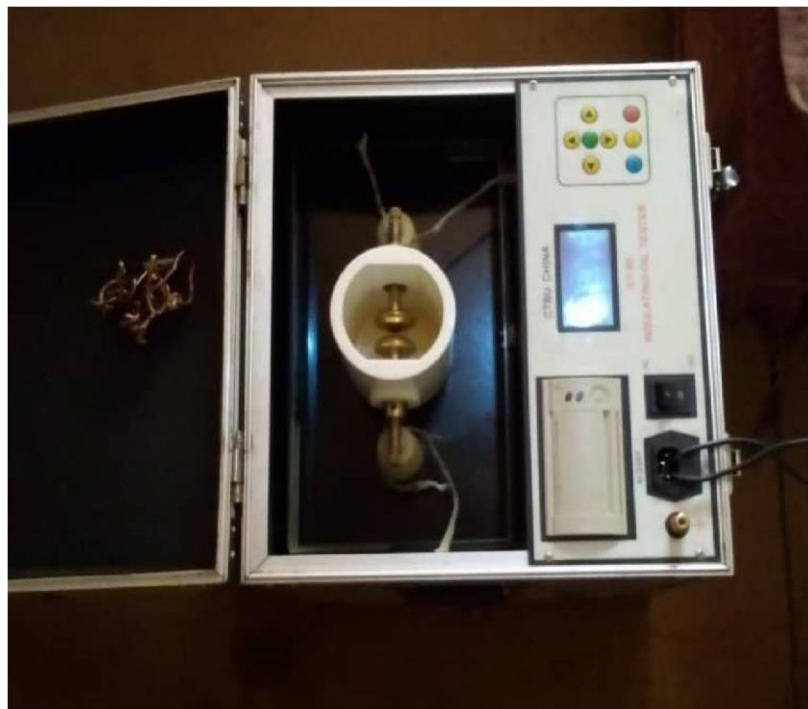
Figure 6: The MEGGER 60 KV Oil Tester Machine used for measuring transformer oil dielectric constant
