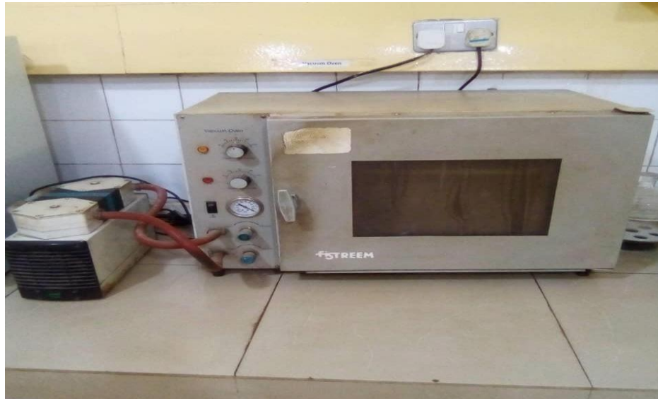
Figure 4: The F-STREEM Vacuum Oven for demoinsturizing water from the oil samples during the determination of moisture content Determiration of the Oil Sludge
