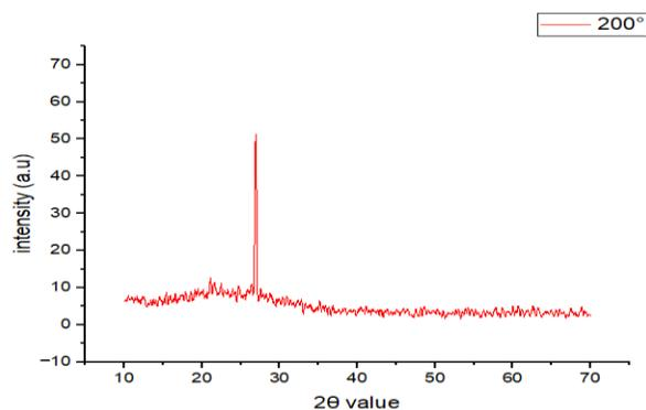
FIGURE 13: XRD result of the ZnO nanoparticles and perovskite materials annealed at 200°C
