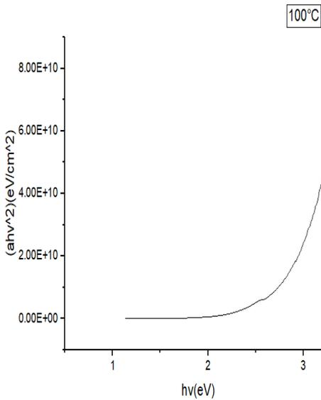
FIGURE 4: Energy band gap of the ZnO nanoparticles and perovskite materials annealed at 100°C and 130°C
