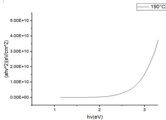
FIGURE 7: Energy band gap of the ZnO perovskite
