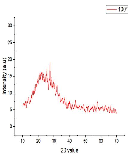
FIGURE 9: XRD result of the ZnO nanoparticles and perovskite materials annealed at 100°C
