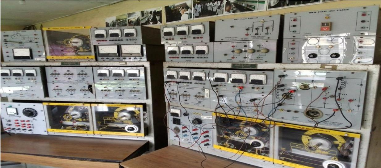
**Figure 4b: Research Laboratory of Pellet Plant of Transients and Speed Control on Conveyor Belt Using a Squirrel Cage Induction Machine [UNIPORT]****5.0: EXPERIMENTAL INVESTIGATION**
