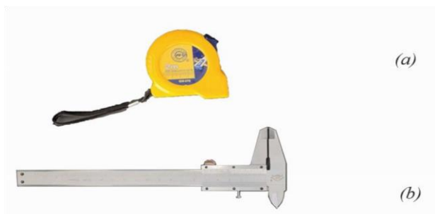
(a)- tape (b)- Vernier caliper Figure 8: Length measuring tool
