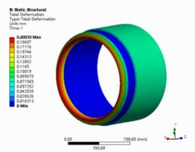
Figure 8: Thermal deformation of the guide sleeve
