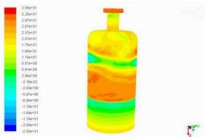
Figure 10: Fluid pressure distribution in the fluid–structure interaction
