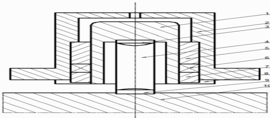
(1) Plunger, (2) cylinders, (3) hinge on the ball, (4) connecting rod, (5) guide sleeve, (6) seal, (7) pressing sleeve, (8) plunger gland, (9) under the spherical hinge, (10) walking beam.
