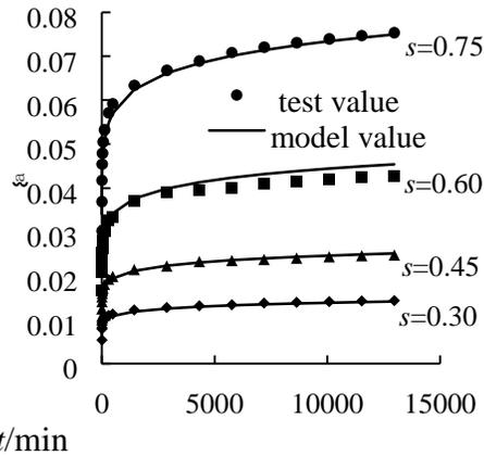
Figure 2: Axial strain  $\epsilon_a$ -time  $t$  curves ( $\sigma_3=300$  kPa)
