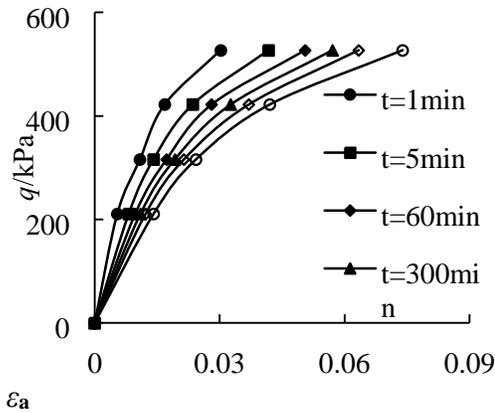
Figure 3: Stress  $q$  -strain  $\epsilon_a$  curves ( $\sigma_3=300$ kPa)
