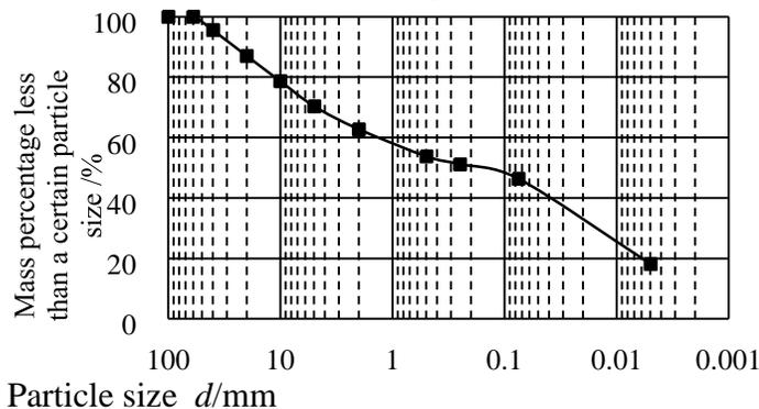
Figure 1: Gradation curve of the sliding zone soils
