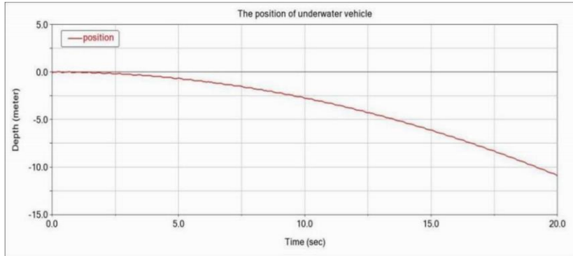
Figure 4: The relationship between the position of AUV's center of mass and time when AUV ascent.
